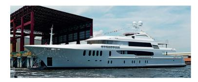
LOA: 196' - Engines: 2 x 2,012 hp Caterpillar 3512B Construction: Steel hull and aluminum superstructure Classification: ABS Maltese Cross A1 Yachting Service, AMS, MCA Naval Architect: Trinity Yachts. LLC
